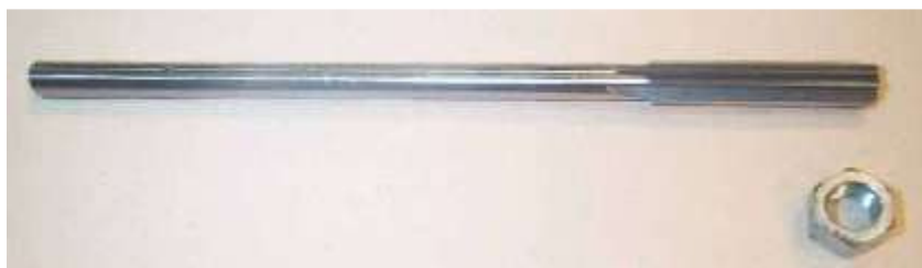
A five-dollar reamer and a 20 cent nut are the main parts needed. Two 8-32 set screws will hold the nut in place.
